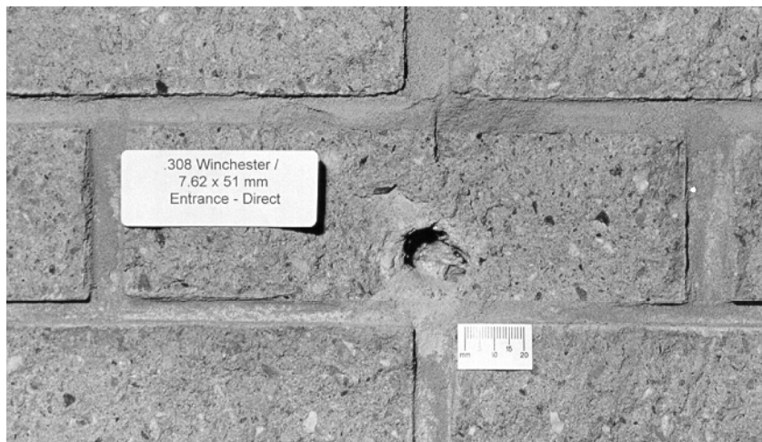
Figure 4 - Damage to concrete brick caused by .308 Winchester
