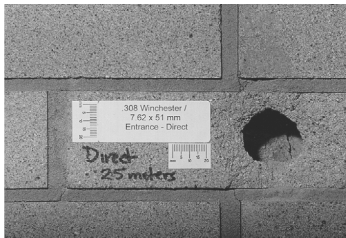
Figure 3 - Damage to clay brick caused by .308 Winchester
