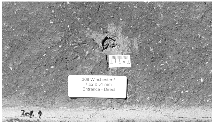
Figure 5 - Damage to red concrete brick caused by .308 Winchester
